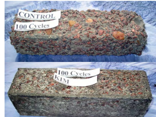
Control concrete vs KIM treated concrete after 100 cycles of freezing and thawing.
