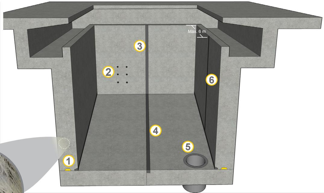
**Krystol®** chemically reacts with water and un-hydrated cement particles to form insoluble needle-shaped crystals that fill capillary pores and micro-cracks in the concrete and block the pathways for water and waterborne contaminants. Any moisture introduced over the lifespan of the concrete will initiate crystallization, ensuring permanent waterproofing protection.
