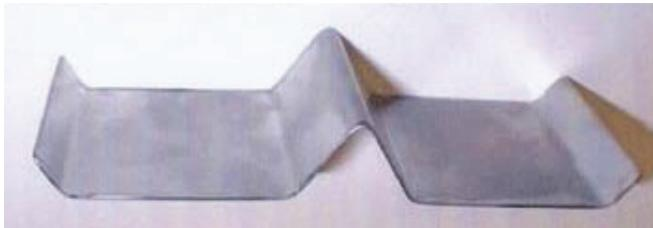
Made of steel, copper, bronze or lead, metallic waterstops are embedded in concrete across joints to form a continuous, fluid-tight barrier. Metallic waterstops are used in specialized applications such as in dams or heavy construction projects where additional strength is required, or where exposure to chemicals or extreme temperatures could damage conventional physical waterstops.
