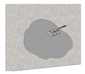
**NOTE:** For deep patches or overlay applications thicker than 13 mm (0.5 in.), mix Krystol Bari-Cote with clean 10 mm (0.375 in.) pea gravel (approximately 4 parts powder to 1.5 parts gravel to 1 part clean water).
